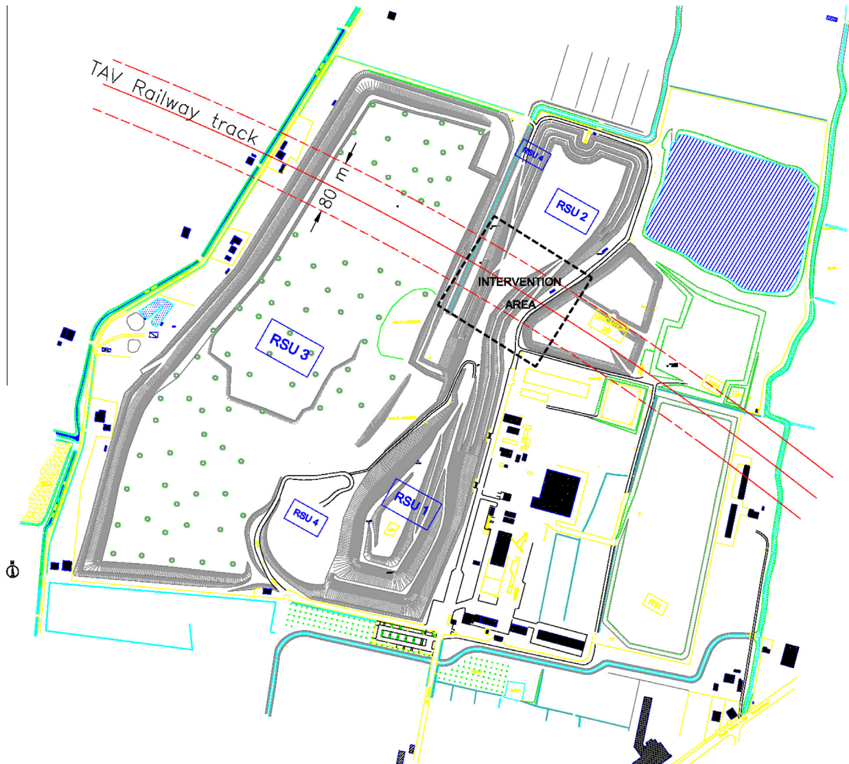
Fig. 1. Layout of the railway track through the landfill site. The black square highlights the area where the aeration took place, in RSU2 landfill.
